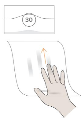
The user moves their hand up the control. The target line and progress fill appear. The center number represents the target speed.
