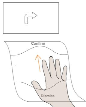
The user swipes on the middle portion of the screen to push the confirm or deny sliders up or down, respectively. The user selects a action by pushing that slider past the edge of the screen.
